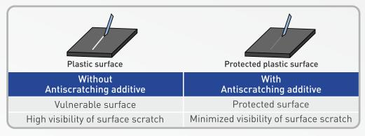
Schematic: Antiscratching additive effectively decreases surface friction by forming a uniform protective additive layer on the polymer surface. Thereby, minimizes the scratch visibility resulting in high-quality surface texture.
