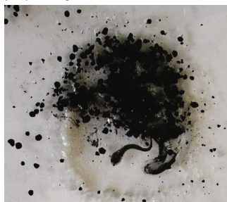
Carbon black in molten polymer granules
