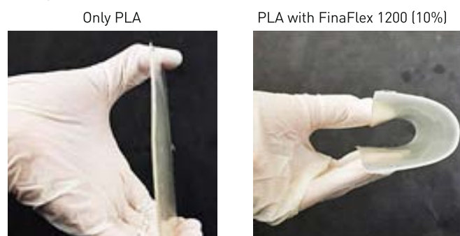
Figure: Bio-plasticizer offering flexibility to the base PLA polymer
